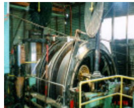
h01879 wattle gully gold mine Fryerstown Road Chewton winding gear 96 db
