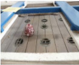
Portland Lifeboat - Wells Patent Lifeboat valves
