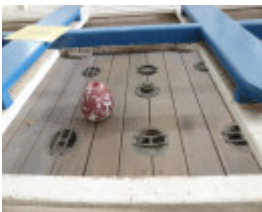
Portland Lifeboat - Wells Patent Lifeboat valves
