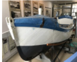
Portland Lifeboat - diagonal planks on other side
