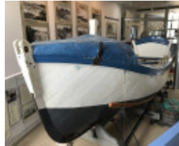
Portland Lifeboat - diagonal planks on other side
